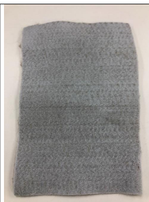
Fig. 6.3.6 Layer of grey geotextile
